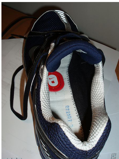
The Nike+iPhone embeds an accelerometer into a pair of sneakers, transforming sneakers into networked objects that create actionable information trails.
